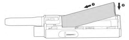
Place the hooks of battery cover to the slots, and then push the battery cover upwards until you hear a click.
